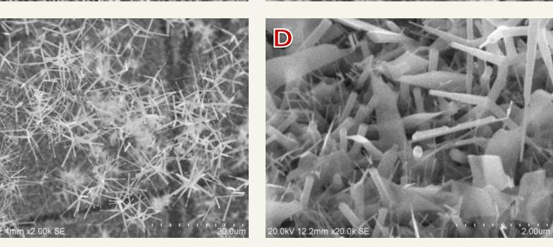
C. Thicker diameters: A. Uniform diameters; inferior alignment; nonnarrow wires grow from textured ZnO film uniform shape and size B. Tetrapod "overgrowth" D. Mix of "nanobelts," "nanorods," tetrapods, extended above
