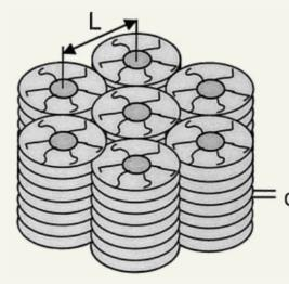
Liquid crystal photovoltaics can self-organize, enhancing charge transfer along axis of orientation [3]
