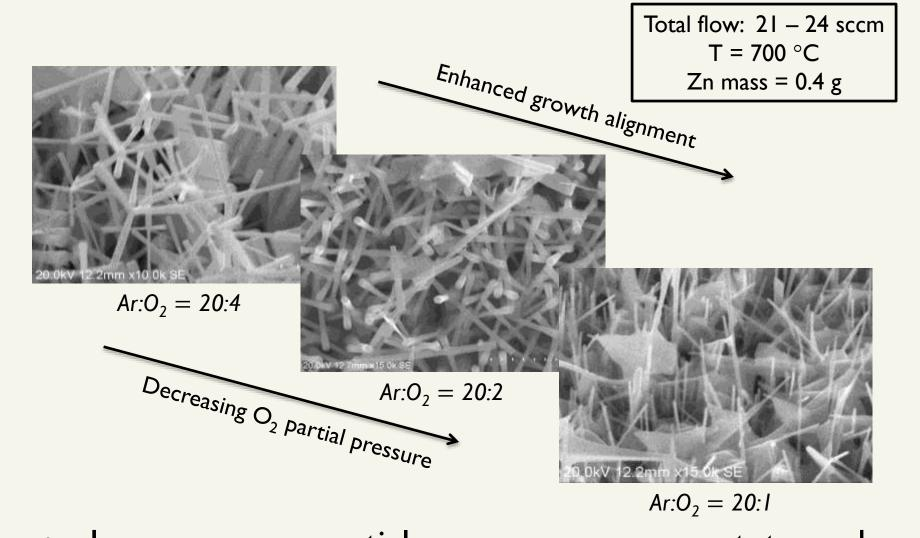
Lower oxygen partial pressure suppresses tetrapod overgrowth and encourages vertical wire alignment
