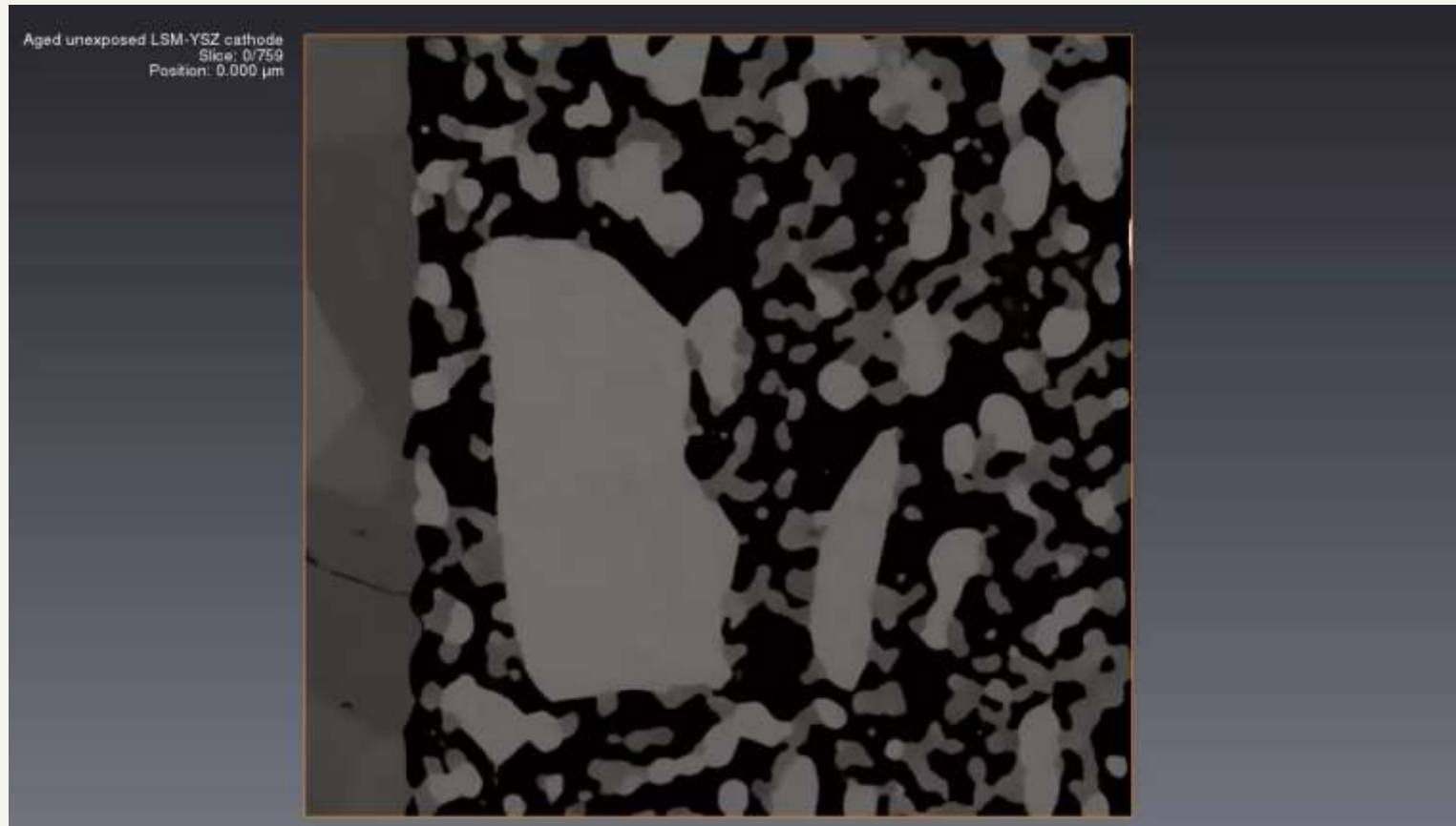
Voxel size: 10 x 10 x 10 nm , EsB signal collected on Zeiss Crossbeam 540, courtesy of Carl Zeiss and Fibics, Inc. HFW: 9.9 \mu\text{m} ; Depth: 8.12 \mu\text{m} ; Total reconstructed cathode volume (excluding electrolyte): 643.11 \mu\text{m}^3
