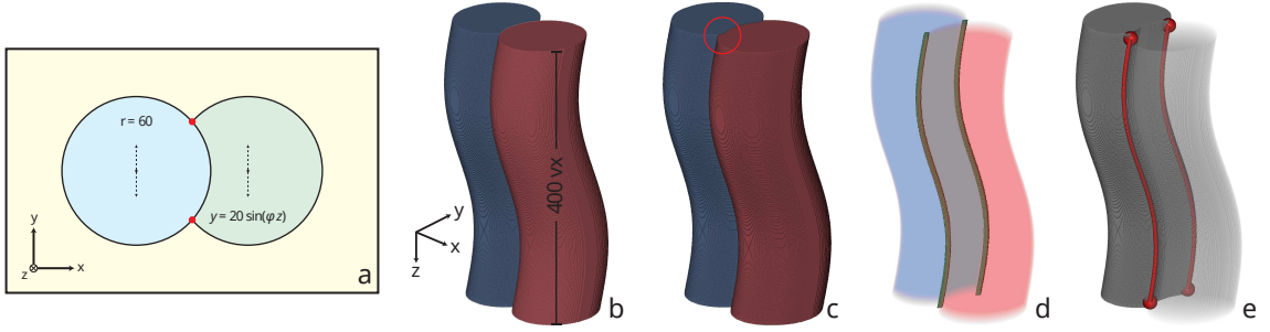
Figure 4.9: Example of TPB test volume and volume expansion calculation method. (a) 2D template used to create test volume. The red dots highlight the TPB points in two dimensions. The positions of the two circles were oscillated together in the y -direction to generate (b), a 3D volume extruded in the z -direction. In this example, \varphi = \frac{2\pi}{400} , such that one period of the sine function was completed over the 400 z voxels. (c) The original surfaces are dilated by four voxels in each of the six neighboring directions, causing the two cylinders to overlap one another by a small amount. Evidence of the overlap is visible in the area circled in red. (d) The overlapping volume of the dilated data is located at the interface between the two phases, as expected. (e) This volume is then skeletonized using typical thinning algorithms to yield the TPB network (shown in red).
